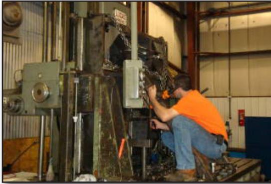
Setting up 6 ft. diameter piece for facing work in horizontal boring mill
