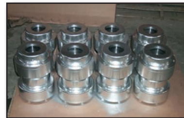
MMW reverse engineered reel spool bearing housings for paper machine
