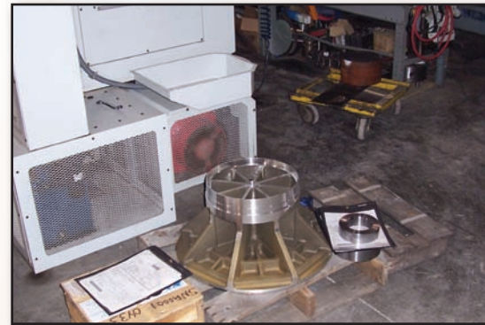
MMW completed titanium base with stainless screen for parts shaker used in reliability testing
