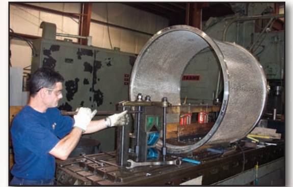
MMW repair / rebuild pulp centri- screen for paper company
