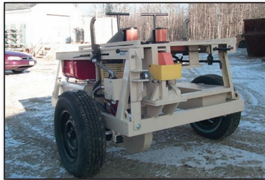
MMW "Ironmaster" portable rebar bender / shear completely manufactured by MMW
