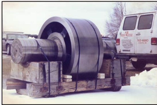
Built / replaced shaft and resurfaced lime kiln trunion
