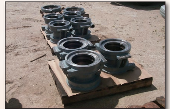
MMW fabricated / machined vessels for cooling chambers in mining industry
