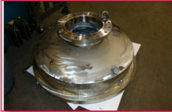
Machined stainless vessel cover 60 inch diameter
