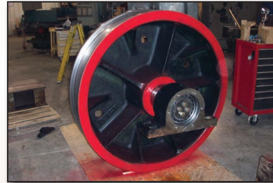
MMW manufactured wood debarker support trunion assembly complete with fabricated bearing housings
