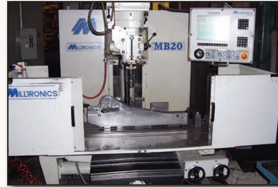
MMW CNC milling machine (1 of 9 CNC Mills) working on titanium material for mold used in molded fabric industry
