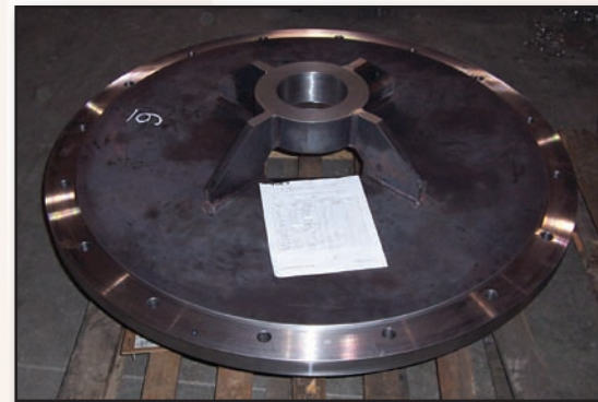
MMW large 6' dia cast/machined end cover for roll
