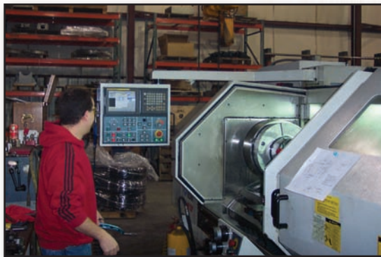
MMW 27" DIA CNC romi lathe (1 of 13 CNC Machines)
